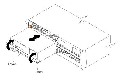
Figure 22. Replacing a power supply and fan unit
